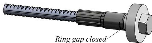
4. If standard M-thread bolt ⑧ is used without a distance sleeve ⑩, the torque moment should be controlled (see Table 10).
