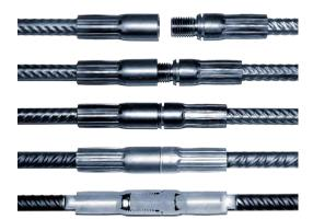
MODIX® Rebar Couplers are building products used to create mechanical connections between ribbed reinforcement bars in cast-in-situ and precast concrete structures. MODIX® consists of prefabricated female and male muffs with M-threads, which are pressed onto the reinforcement bars. This system provides high production speed with reliable quality. A unique visual inspection system makes the assembly process both fast and safe.
